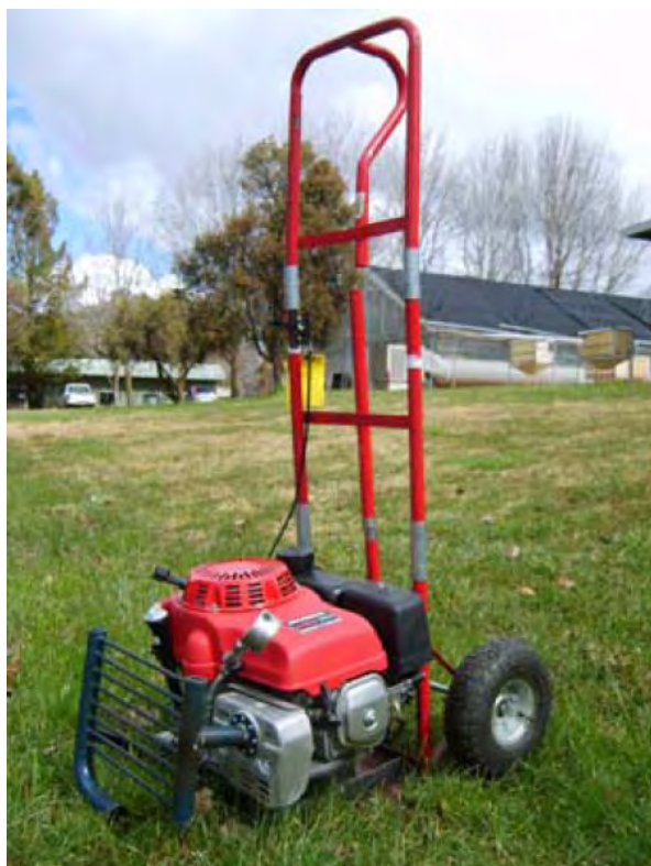
Prototype CO pressure fumigators
